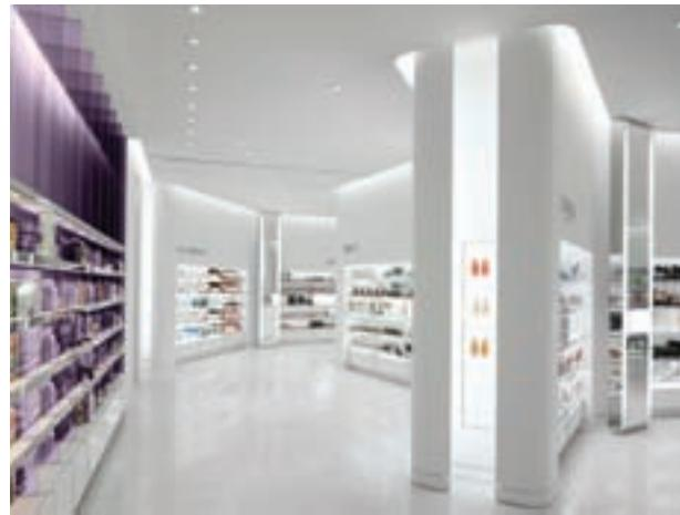
Fluorescent striplights incorporated into full height mirrors provide customers with a flattering, low-glare light quality consistent with displays at which the product was initially selected. High-CRI 3500K T5 fluorescent lamps are used consistently in shelves, coves, and at mirrors.
