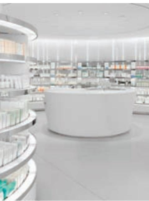
Animated vertical linear arrays of white LEDs are embedded in the white, translucent walls of the skincare area. The LEDs are individually programmed to stream down the wall in a pattern reminiscent of rain.
