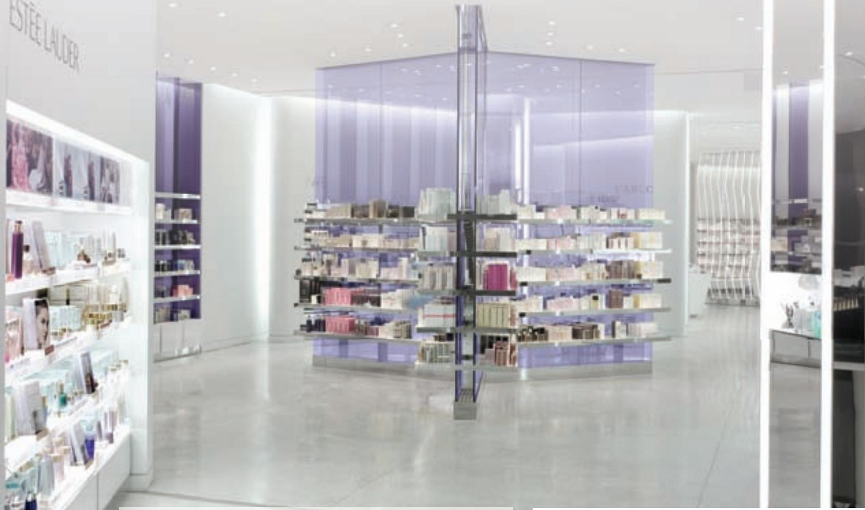
Downlighting was reduced by generating most of the ambient light via localized merchandise lighting. RSA Accurus adjustable pinhole downlights are arranged in graphic patterns, emphasizing circulation routes through the space, and are adjustable for highlighting freestanding and feature displays. The pinhole aperture reduces ceiling glare, enhancing the impact of displays.
