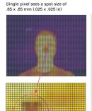
If you set up a  $640 \times 480$  resolution infrared camera about 1 meter from a subject, the resulting image plane would be  $418 \times 312$  mm ( $16.45 \times 12.28$  in). Therefore, a single pixel would have a spot size of  $.65 \times .65$  mm ( $.025 \times .025$  in).
